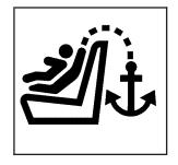
To assist you in locating the top tether anchors, the top tether anchor symbol is located near the top tether anchors.
